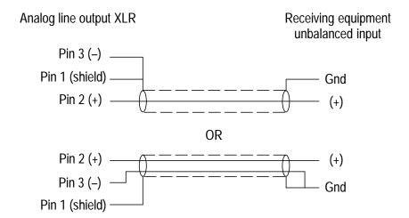
Figure 40: Connecting to an unbalanced input
